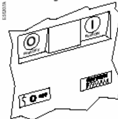
Circuit breaker open and discharged
