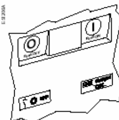
Circuit breaker open, charged and not "ready to close"
