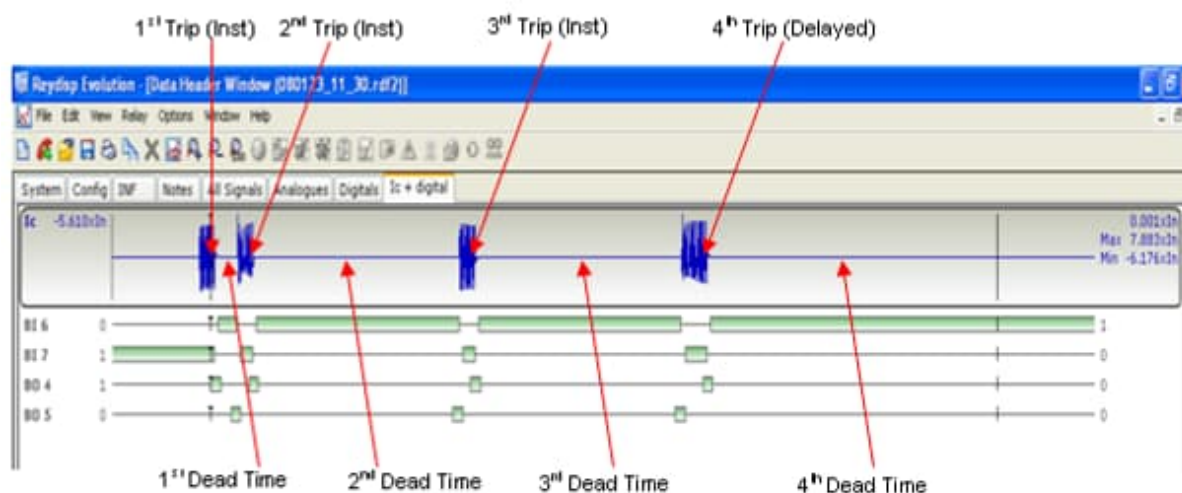
Figure 4-1 Typical AR Sequence with 3 Inst and 1 Delayed trip
