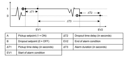
**NOTE:** To prevent filling the alarm log with nuisance alarm trips, the digital alarm is automatically disabled if the digital / status input changes state more than 4 times in one second or more than 10 times in ten seconds. In this case, you must re-enable the alarm using the display or ION Setup.
