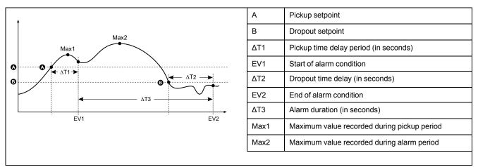
The meter records the date and time when the alarm event starts (EV1) and when it ends (EV2). The meter also performs any task assigned to the event, such as operating a digital output. The meter also records maximum values (Max1, Max2) before, during or after the alarm period.
