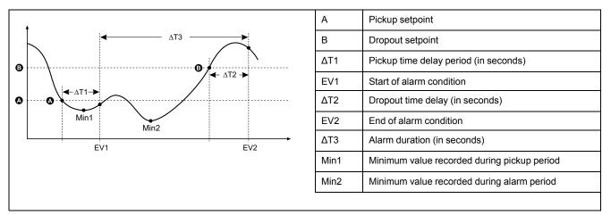
The meter records the date and time when the alarm event starts (EV1) and when it ends (EV2). The meter also performs any task assigned to the event, such as operating a digital output. The meter also records minimum values (Min1, Min2) before, during or after the alarm period.
