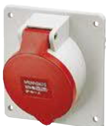
Panel mounted receptacle 63 A: X-CONTACT, standard flange dimensions, uniform fixing hole spacing, 15° inclination for 16 A and 32 A, 20° inclination for 63 A
