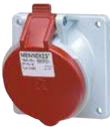
Panel mounted receptacle screwless, with TwinCONTACT, standard flange dimensions 85 x 85 mm, 20° inclination, optional fitted with auxiliary contact
