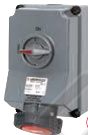
Wall mounted receptacle X-CONTACT, highly resistant to chemicals, highly heat resistant contact carrier, nickel plated contacts, with mechanical DUO-interlock
