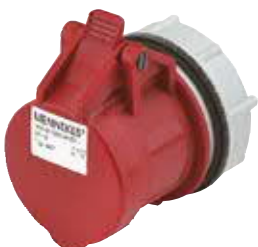
Panel mounted receptacle RAPIDO screwless, with TwinCONTACT, with central locking system, round flange for central fixing, diam. 70 mm
