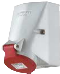
Wall mounted receptacle screwless, with TwinCONTACT, suitable for through wiring, internal fixing, enclosure base can be turned 180°
