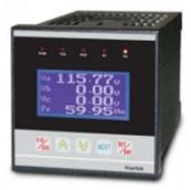
PF-3150 Power Quality Meter uses a 3Ø power measurement chip as it's core processor, it is able to measure all power units (V, I, F, P, Q, S, PF, QE, SE). The PF-3150 is equipped with 2 relay contact output which could be set to action upon user-determined values of voltage (V), current (I), Power (W), Power factor (PF) and Power Demand. Also available are 2 sets of transistor output with pulse/KWh and pulse/KVARh output function.
