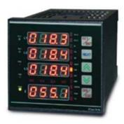
PF-3350 Power Quality Meter uses a 3Ø power measurement chip as it's core processor, it is able to measure all power units (V, I, F, P, Q, S, PF, QE, SE). The PF-3350 is equipped with 2 relay contact output which could be set to action upon user-determined values of voltage (V), current (I), Power (W), Power factor (PF) and Power Demand. Also available are 2 sets of transistor output with pulse/KWh and pulse/KVARh output function.
