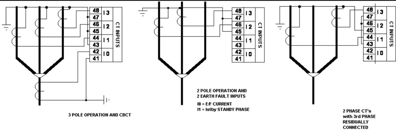
In the residual earth connection it may be a requirement to addition a stabilising resistor in the earth return leg, this is generally only required when EF protection is set at a low threshold and fast operating time.
