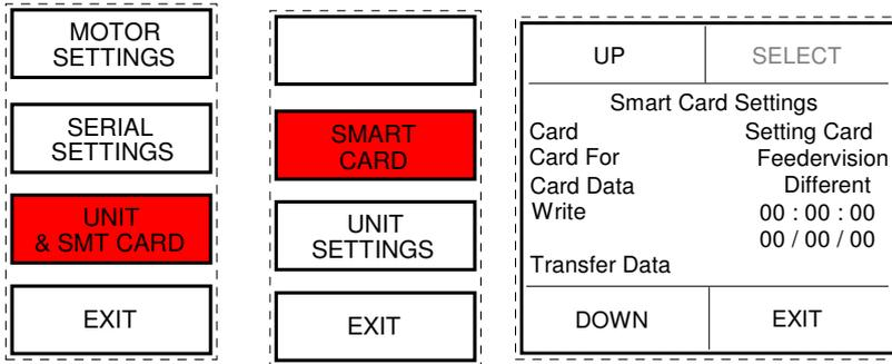
The Smart Card is a removable eeprom memory card which can be supplied with FV2 on request.
