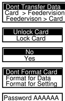
The Card detail is displayed on the first two lines, the card data indicates whether the parameter settings both on the card and those programmed into the relay concur with each other. Any single setting change causes Compare Fail to be displayed across the screen.
