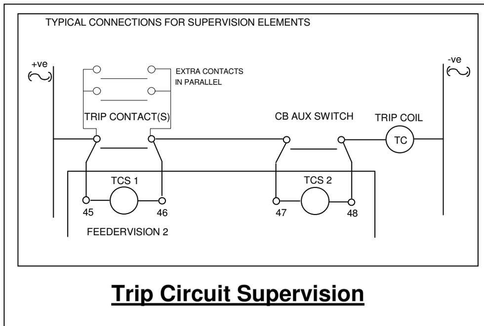
The TCS element consists of two input circuits and two dedicated change-over contact output relays operating in tandem. As the TCS board does not interact with the main relay processor one of the digital outputs provided by the Trip Circuit Supervision should be fed back into the FV2 or EFV2, as an External Fault input. The other output can be used to drive an indication lamp or other such application.
