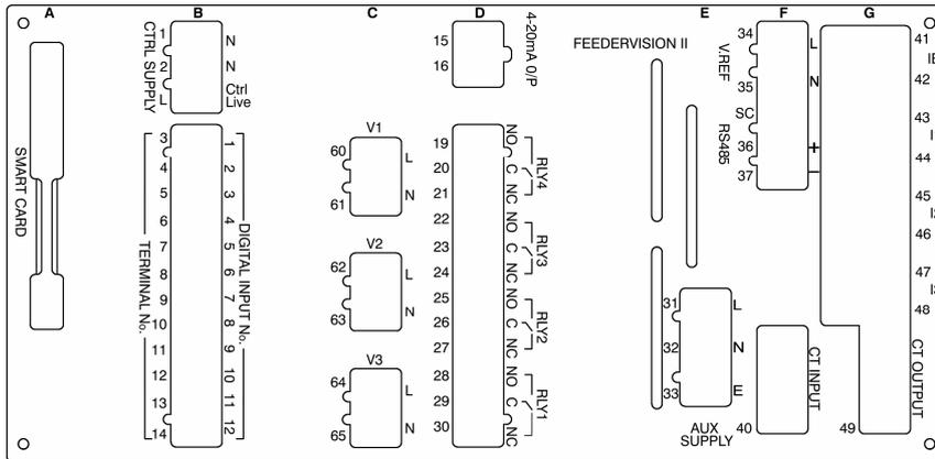
FV2 with 4-20mA backplate layout with CT card
