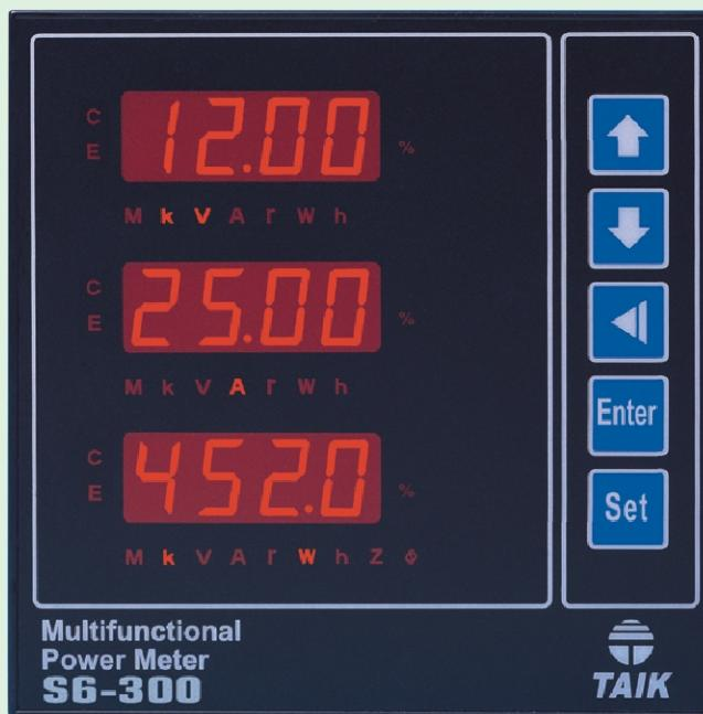
effectively monitored by relay contactors, analog outputs and a convenient digital output. This meter is equipped with serial communication for a remote control through standard interface either RS-485 or RS-232. Meanwhile, S6-300 also utilizes the modbus communication protocol to transmit all electrical information in a digital form to PC, PLC, SCADA and even a display repeater.
