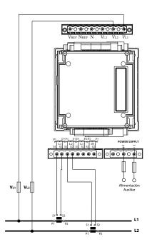
Measurement in single-phase system with or without voltage transformer
