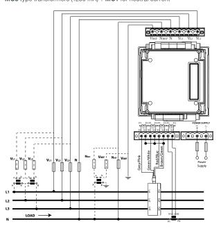
Direct phase-phase measurement with current transformers
