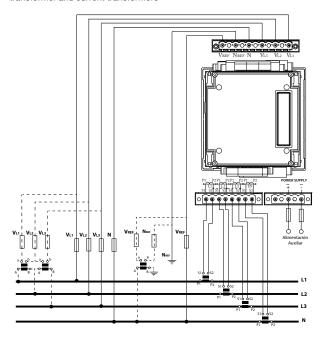
Three-phase measurement, with or without voltage transformer and **MC3** type transformers (1250 mA) + **MC1** for neutral current
